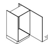
**GK Appliance housing for refrigerator / recess 1025 mm**
