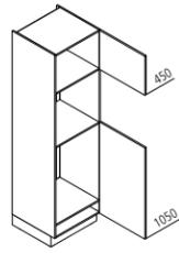
**GKB** Appliance housing for refrigerator and oven / recess 880 mm
