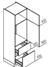
**GKZ Appliance housing for refrigerator / recess 880 mm**
