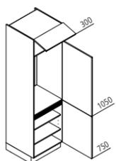
**GK Appliance housing for refrigerator / recess 1025 mm**
