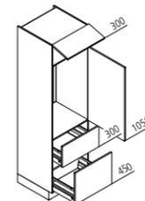
**GKZ Appliance housing for refrigerator / recess 1025 mm**
