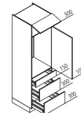
**GKAK Appliance housing for refrigerator / recess 1025 mm**
