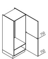
**GK Appliance housing for refrigerator / recess 1225 mm**
