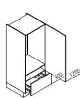
**GKA Appliance housing for refrigerator / recess 1025 mm**
