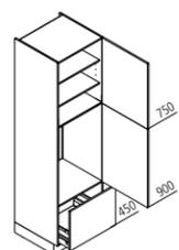
**GKA Appliance housing for refrigerator / recess 880 mm**
