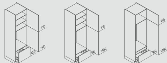
By way of example, an appliance housing for a refrigerator in 2100 mm height with recess heights of 880, 1025 and 1225 mm (from left to right).
