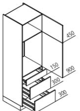
**GKAK Appliance housing for refrigerator / recess 880 mm**
