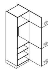
**GK Appliance housing for refrigerator / recess 880 mm**
